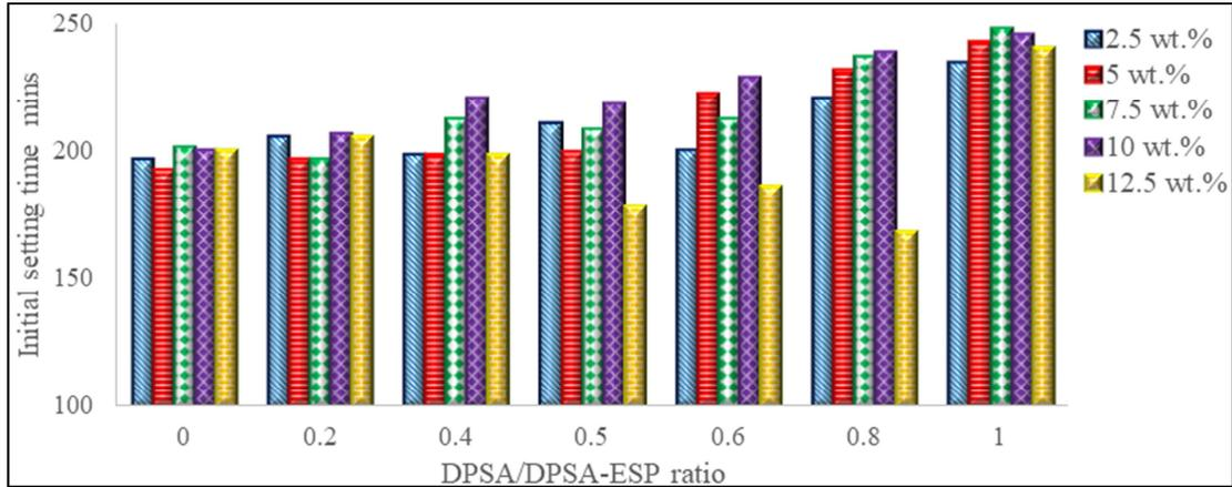
Figure 2. Variation of DPSA/DPSA-ESP ratio on the Initial setting time of cement blends at various cement replacements.
