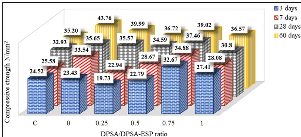
**Figure 5.** Variation of curing age on the mortar compressive strength at various DPSA/DPSA-ESP ratio for 2 wt. % cement replacement.
